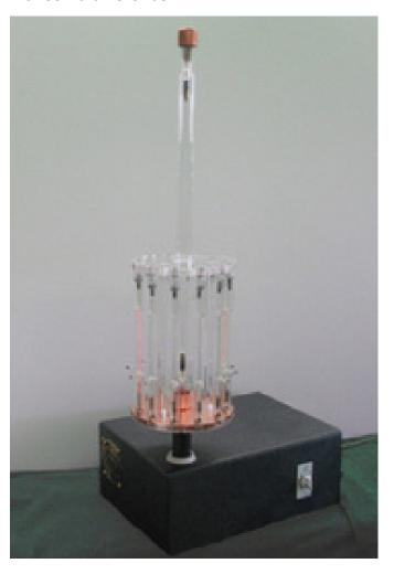
The number of photons emitted depends on two variables, the voltage applied and the amount of gas. While its true that longer tubes will contain more gas, the units that use the longer tubes, TESLA ENERGY LIGHTS and SEAD 3000/6000 have much smaller tesla coils and hence much weaker voltages. So the actual number of photons emit may or may not be more than the smaller tubes on the higher voltage devices.
