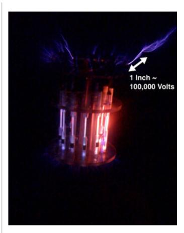
A general rule of thumb is that one inch of corona discharge (or spark) of the unit is equal to about 100,000 volts.
